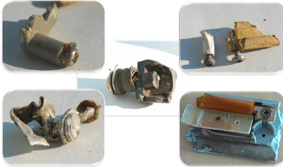
Figure 19 Some examples of bolts/rivets from dissimilar (incompatible) materials.
