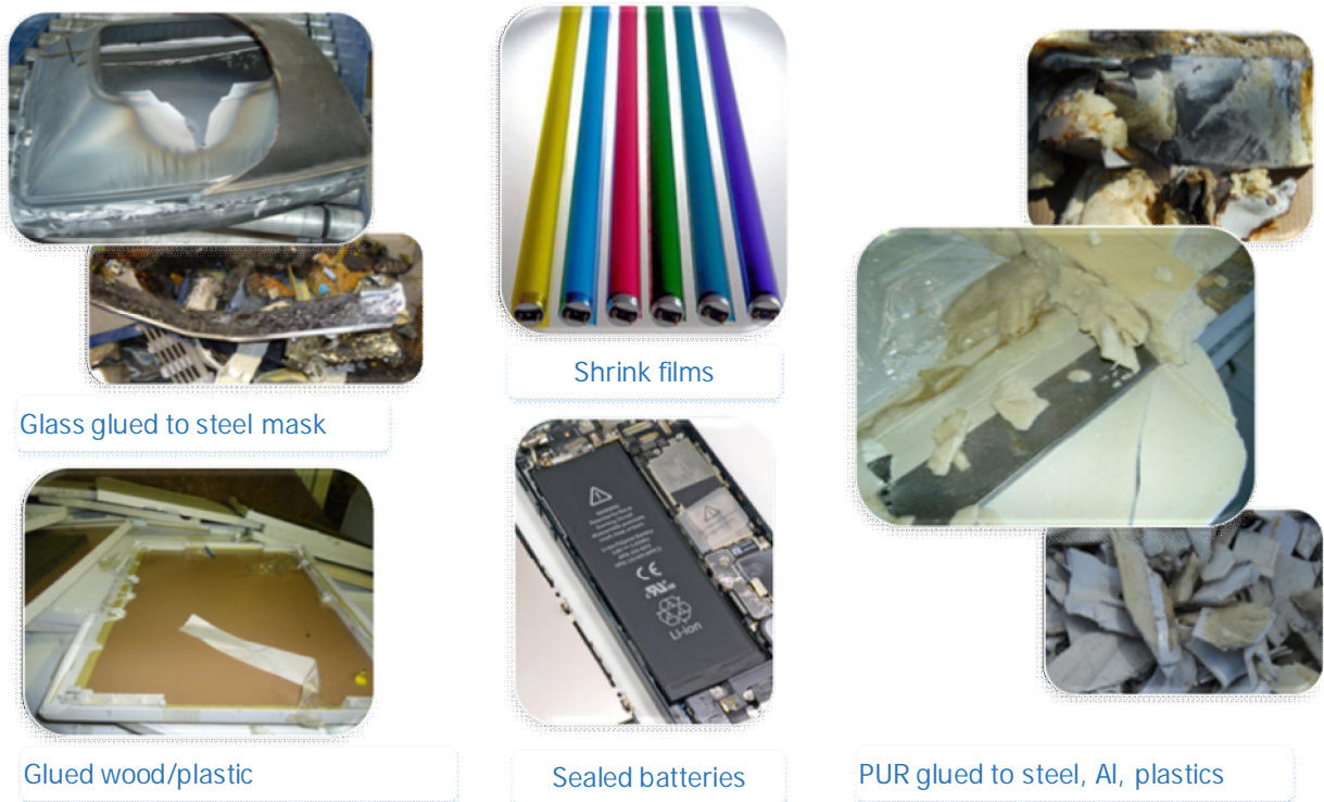
Figure 20 Non-reversible adhesives for incompatible & undesired material combinations causing problems and material losses during liberation, sorting and final treatment processing.
