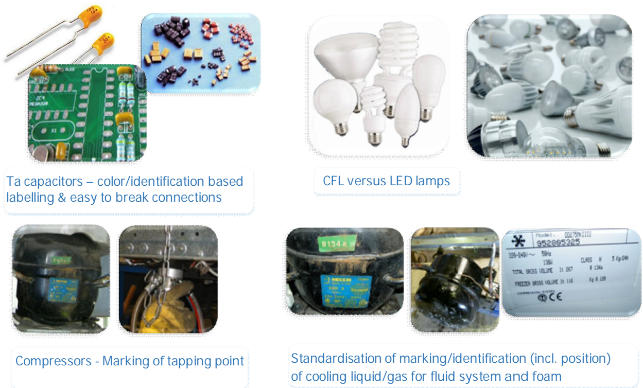
Figure 18 Some examples of requirements and suggestions for labelling and marking for Waste stream Sorting and (Automated) Disassembly & Sorting (including input from recyclers/pre-processors).
