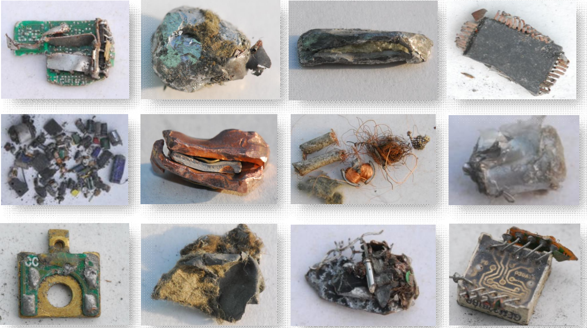
Figure 21 Particulate quality (determining recycle quality and recovery/losses) as a function of design. An impression of unliberated and multi-material particles as found in various WEEE recycles.
