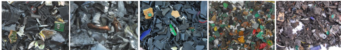
Figure 8 Recyclate quality from WEEE product due to inevitable imperfect separation & liberation - particles, distributions in which (a) ferrous recyclate; (b) aluminium recyclate; (c) plastics recyclate.; (d) Printed Circuit Board recyclate; (e) residue fraction.
