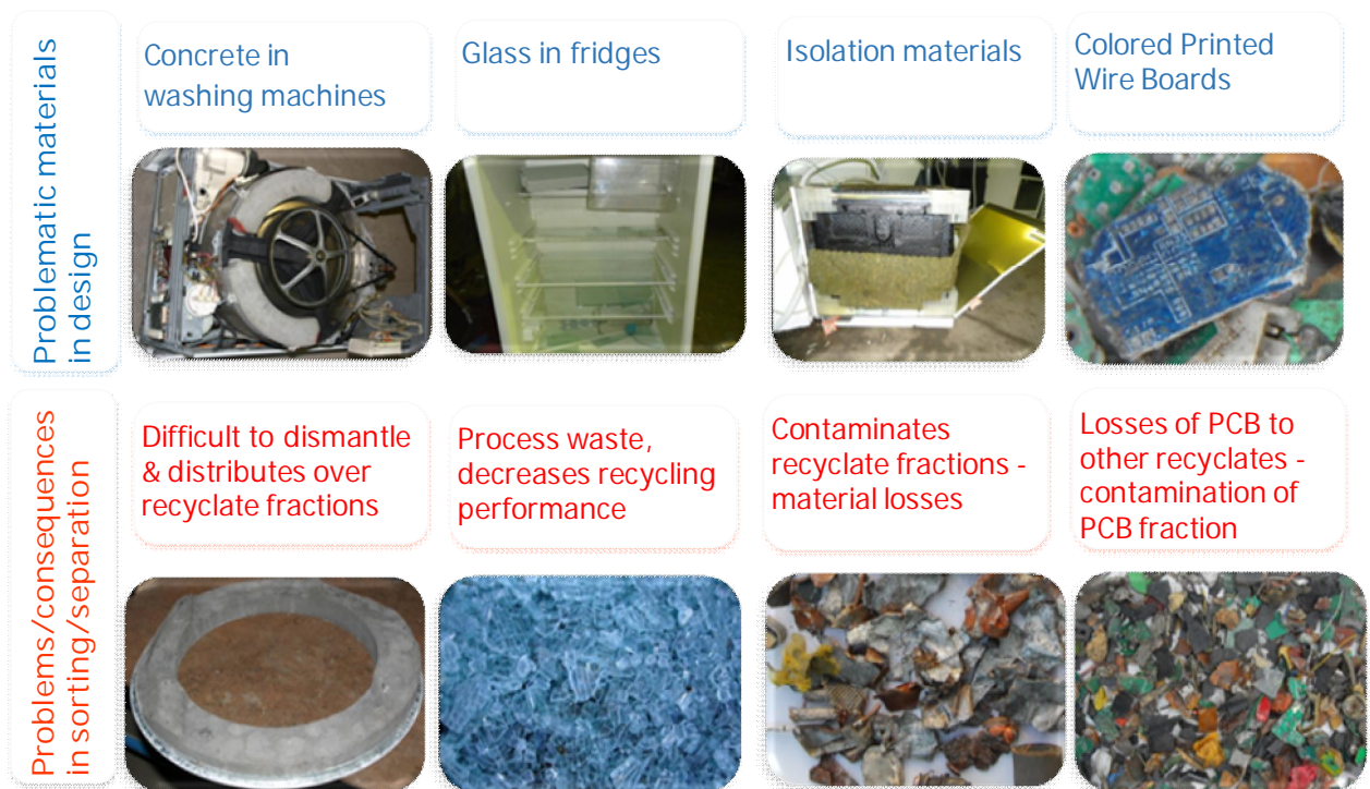
Figure 15 Some examples of materials applied in WEEE and the problems arising in sorting/separation as a consequence.
